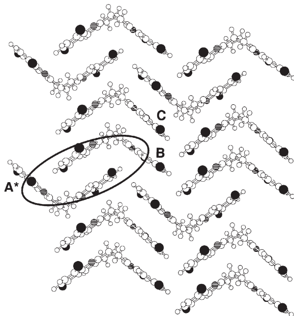
FIGURE 10 Projection view in the ab plane of a layer in the (\mathbf{5})_3 \cdot (\text{chloro(chlorobenzene)})_2 structure, with one PHD unit highlighted by an ellipse. Here, the host molecules form A^* - B PHD units that are linked through C molecules by means of OFF interactions. (The adjacent layers contain the A , B^* and C^* host molecules). The chlorobenzene guests are omitted from this figure for clarity.
